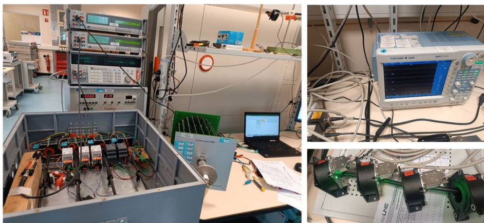
Calibration of the EV charging station power AC reference measurement setup at LNE's laboratories.
