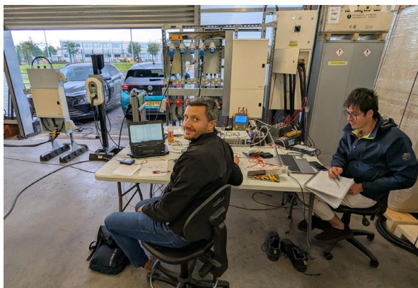
The Universities of Strathclyde and UPV/EHU during a measurement campaign at PNDC (UK) to assess grid impedance and disturbances associated with EV charging stations.
