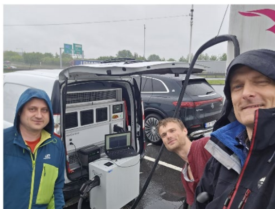
CMI institute on-site verification of DC metering accuracy in EVCSs.
