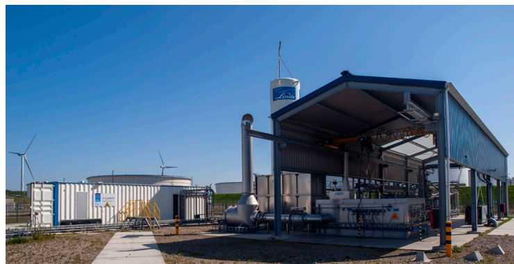
Figure 2. VSL LNG flowmeter calibration facility.
