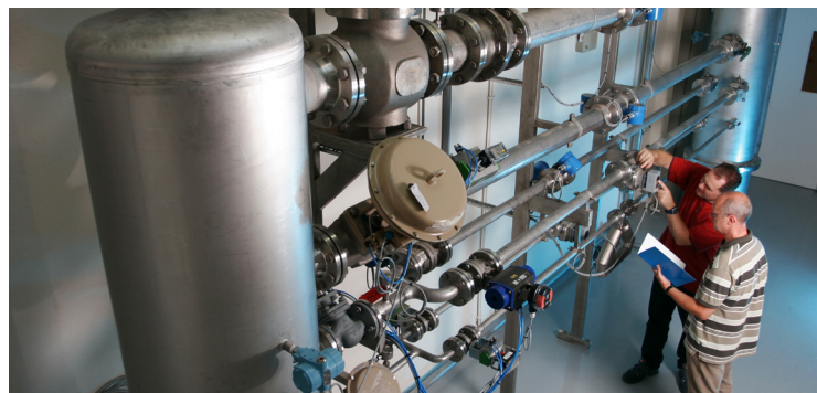
Figure 1. Master meter section in VSL flowmeter calibration facility.
