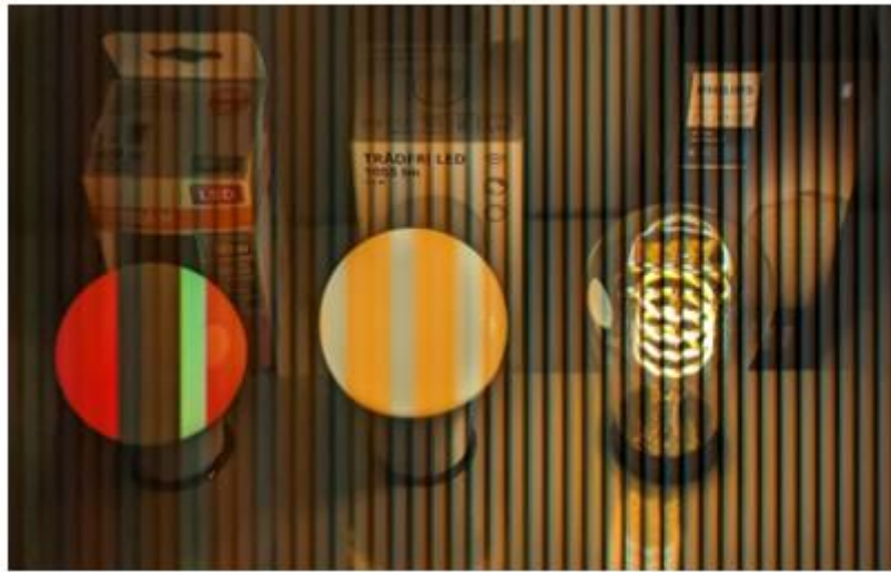
Figure 8: photo of smart LED-based lamps rendering TLM artefacts by the rolling shutter.
