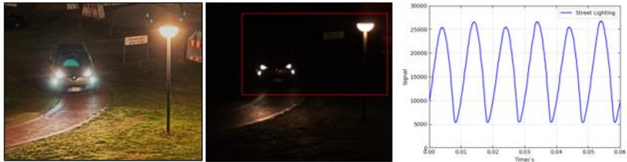
Figure 10: photo of a night-time outdoor scene including a car and a HID-based luminaire (left), still image of the high-speed camera indicating the area of interest covering 1184 \cdot 584 pixels for which a sequence at 8000 fps with an integration time of 122 \mu\text{s} was captured (centre), and extracted waveform signal corresponding to the HID-based luminaire (right).
