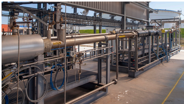
Figure 2. Flowmeter under test (MUT) section of VSL's LNG calibration facility.
