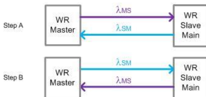
Figure 7. Schematic diagram of the fibre delay asymmetry calibration
