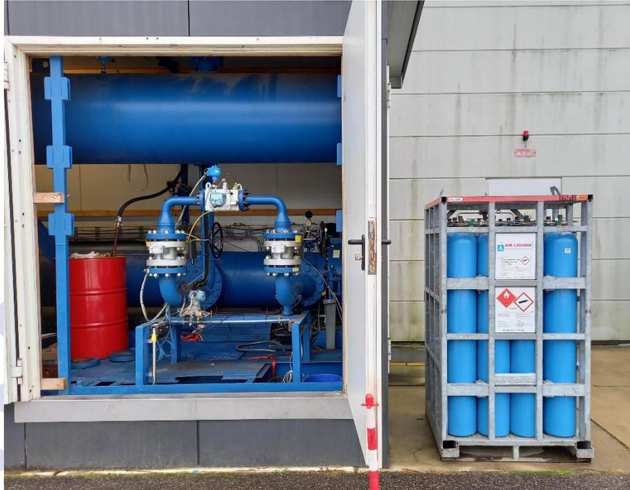
Figure 1. MuT mounted on VSL's GOPP, accompanied by hydrogen gas cylinders.
